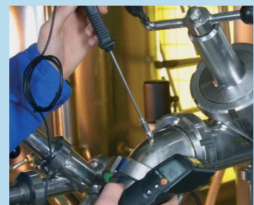
Connection for external temperature probes (testo 830-T2)
