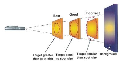
For accurate IR temperature measurement, the target should be larger than the instrument's field of view, or spot size. If the spot size is larger than the target, energy emitted from the background or surrounding objects may also be measured and reduce accuracy.
