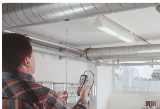
Using the testo 425 to set the air input in a kitchen
