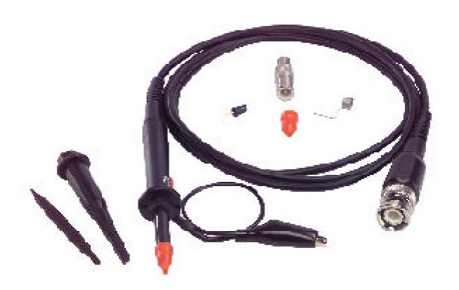
General purpose replacement probe with 3-position switchable attenuation, x1, x10 and Ref. 100MHz @ -3dB x 10 position, 10M $\Omega$  impedance (1M $\Omega$  scope input), 16pF capacitance, <3.5ns risetime. 300 V CAT II, 1M $\Omega$  impedance (scope input), 90pF capacitance, 58ns risetime. Ref position disconnects the probe tip and grounds the scope input. 1.2m cable length with low-naise compensation, 10-35pF, in BNC box.
