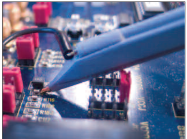
Probe directly on surface mount components like resistors or capacitors with the Discrete SMD Tip. Use this tip with any of the ground leads, like the flexible Long Right Angle Lead shown here.
