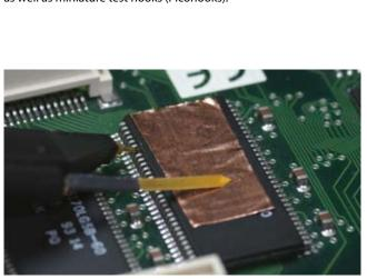
Very short ground connections can be established with the ground blade and the copper pads – for signal true measurements on ICs.
