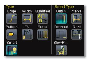
The advanced triggering of the MSO Xs-A goes well beyond the basic edge trigger and digital pattern trigger that many MSOs offer. Advanced triggers like runt and dropout and slew rate help find abnormal signals. The Qualified AB trigger can be used to connect multiple trigger events together.
