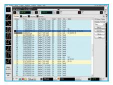
Fill the entire display with compact protocol information. The protocol viewer shows index number, time stamp, and data content for each serial packet. Listing content can be saved to a .csv or .txt file for off-line analysis or documentation. Use search capability to quick navigate through an acquisition.
