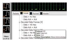
Details tab breaks the packets into easyto-read textual fields. Hovering shows additional detail.
