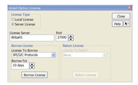
Sharing the application across multiple instruments? Server-based licensing allows users to borrow an application license for a specified period of time.
