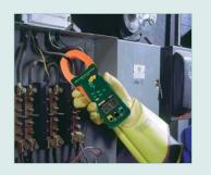
Large jaw size for high current measurements
