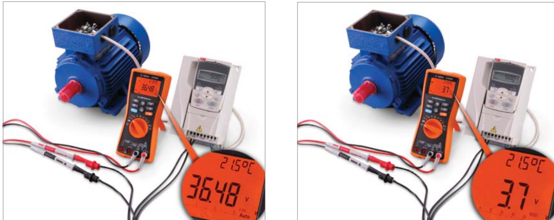
Figure 1: U1272A helps you identify the presence of stray voltage on a disconnected wire running parallel with the wire powering up the VFD to an industrial motor. The image on the right shows the U1272A in low impedance mode.
