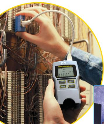
Users can quickly move through Voice, Data, Video/Security networks, testing all wiring types using the same tester.
