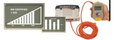
DECODE A HUB, SWITCH AND PC'S CAPABILITIES AND SIGNAL LEVEL. GO "INLINE" BETWEEN TWO DEVICES FOR THE "NEGOTIATED" SPEED.
