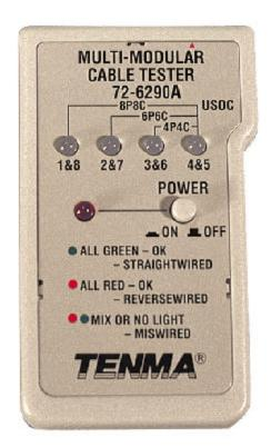
Multi-Modular cable tester for USOC4, USOC6, USOC8 cables with RJ-45, RJ-12 and RJ-11 connectors
