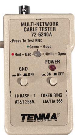
The multi-netwrok cable tester quickly tests by scanning the wires continuity, miswiring and polarization in network cales. Tests Ethernet 10Base-2(BNC),
