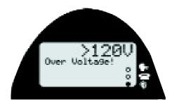
The PE830 automatically checks for high voltages and currents..
