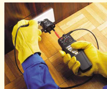
Phase rotation direction is defined by a TT, TN, or IT neutral system due to an innovative 2-wire method. This test operates on generator sets.
