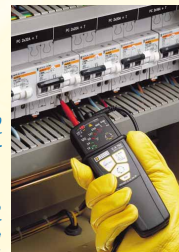
Used together, the C.A 751 + C.A 760 create a resistive phase-earth link for safely testing a 30 mA circuit breaker at 230 V AC.
