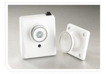
Electromagnetic Fire Door Holders are designed to hold open Fire Doors in any areas where easy access is essential, and can be used in conjunction with any suitable fire alarm systems. When an alarm is triggered, power to the door holder is cut, allowing the fire door fitted with it's standard closing mechanism, to shut automatically. Type 87 door holders are fitted with an integral manual release button, allowing the door to be closed without operating the fire alarm.
