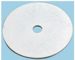
Steel mudguard washers. Also known as penny washers, the oversize outside diameter gives extensive spread of the clamp load. Bright Zinc plated.
