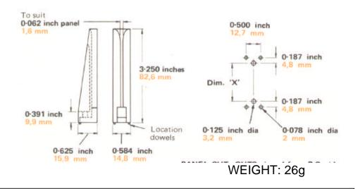
PANEL CUT-OUTS viewed from P.C. side Dimension 'x' to be fixing centres of any P.C. connector Location dowel holes to be within 0.05mm dia of true position
