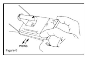
Carefully press the door and chassis in vertically opposite directions until the catch is released. Do not pull the door and chassis apart without first releasing the catch.
