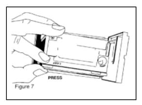
Fit a replacement cartridge, ensuring that the paper lies between the ribbon and the steel printer platen.
