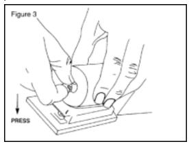
Thread the new roll past the retention button onto the spindle with the paper unspooling in an anticlockwise direction when viewed from the open end. (See Figure 4). Press the paper feed actuator arm (at upper left in data mode) until the mechanism grips the paper and pulls it through to the front of the printer. (See Figure 5).
