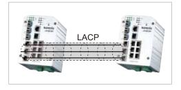
technology. Now, there is no recovery time when failures occur. The JetNet 4010 provides a simple and easy way to aggregate port bandwidth into Rapid Super Ring.
