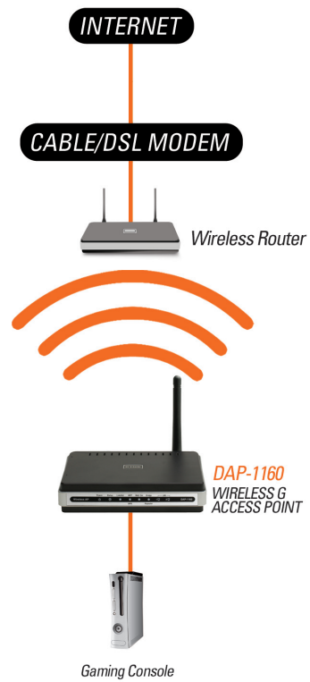
Ethernet-enabled gaming console using the DAP-1160 as a wireless interface to access the Internet
