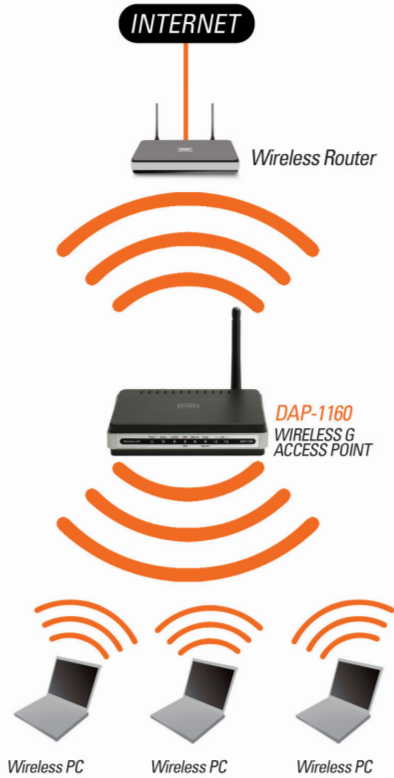
Extending the wireless coverage of a wireless router using the DAP-1160
