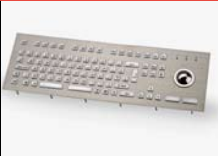
Alphanumeric keyboard, top mounting, 91 keys, stainless steel track ball, 6 rows/MF2, 2 clicks, PS2 and USB output types, English, German, French and US English layouts
