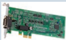
PX-387: PCIe 1xRS422/485 1MBaud Opto Isolated
