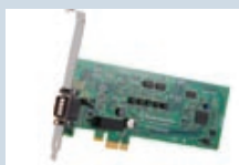
PX-387: PCIe 1xRS422/485 1MBaud Opto Isolated
