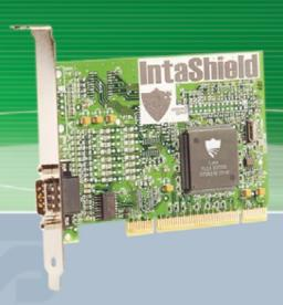
This card provides 1 industry standard 9 pin RS232 serial COM port in a single PCI slot. As PCI is fully Plug & Play compatible the operating system or BIOS automatically configures the card ensuring conflict free installation.
