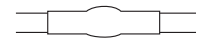
3. Apply heat to the connector until solder and adhesive flows and tubing recovers. Allow the connector to cool.
