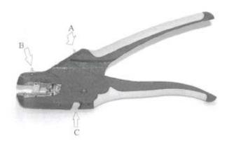
The D01627 has been designed to remove insulation from wire and cables, ideal for installation electricians. The design of the tool enables the user to strip cable of 6mm<sup>2</sup> (10AWG) down to 0.08<sup>2</sup> (27AWG) with an easy action gripping pad adjuster (A) and blade depth adjuster (B); providing in the one tool what was previously only available by having several. The tool also has a cut off blade (C) handling cable up to 6mm<sup>2</sup> (10AWG) stranded copper conductor.
