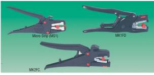
A range of automatic wire strippers to cover cable sizes  $0.25 \rm mm^2$  to  $6.00 \rm mm^2$ . They all operate using a unique system of self adjusting multiple blades which slice cleanly through the insulation but then form around the conductors to give a clean cut without causing any damage.
