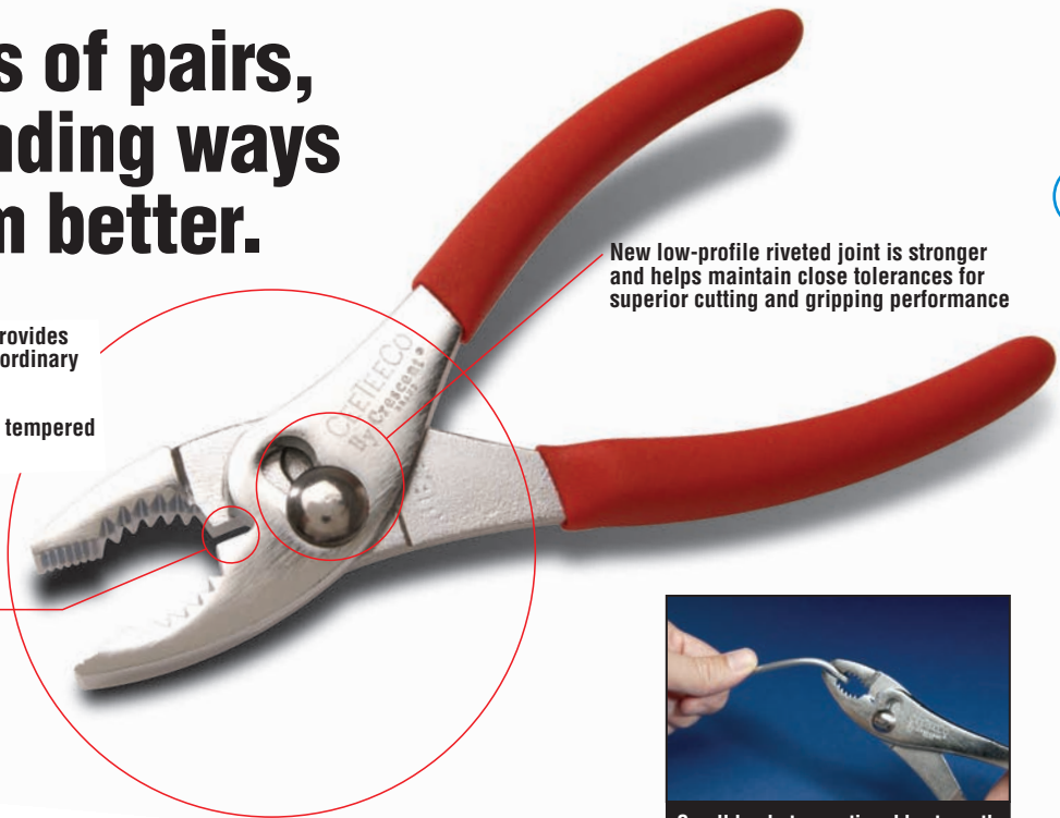
Small land at nose tip adds strength and reduces chipping when pulling
