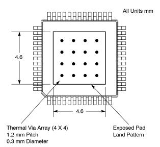
Figure 7. Recommended Thermal Land Pattern
