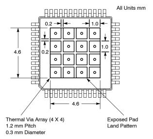
Figure 8. Recommended Solder Mask Openings
