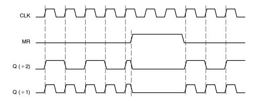
Figure 4. Master Reset (MR) Timing Diagram
