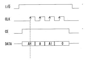
If the AH="1" is set, the last 4-bit of the input data is only effective and written-down to the system control register.
