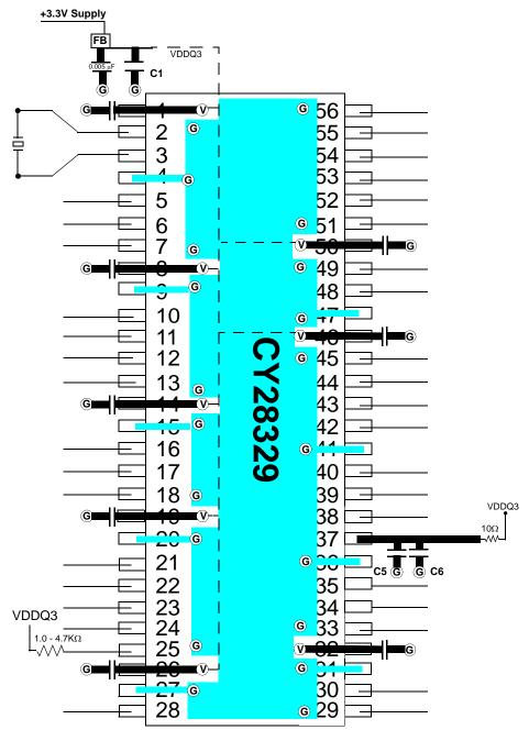
FB = Dale ILB1206 - 300 or 2TDKACB2012L-120 or 2 Murata BLM21B601S Ceramic Caps C1 = 10–22  $\mu\text{F}$  C2 = 0.005  $\mu\text{F}$  C5 = 0.1  $\mu\text{F}$  C6 = 10  $\mu\text{F}$  G = VIA to GND plane layer \$V\$ =VIA to respective supply plane layer Note: Each supply plane or strip should have a ferrite bead and capacitors
