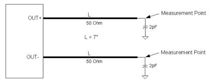
Figure 3. 0.7V Differential Load Configuration
