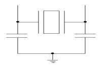
Figure 1. Crystal Capacitive Clarification
