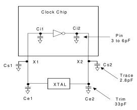
Figure 2. Crystal Loading Example
