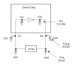
Figure 2. Crystal Loading Example
