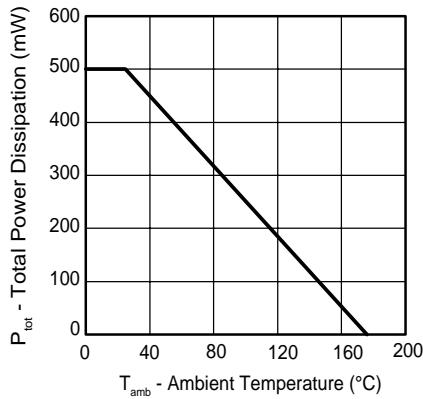
Figure 1. Total Power Dissipation vs. Ambient Temperature
