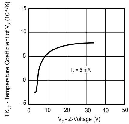
Figure 4. Temperature Coefficient of Vz vs. Z-Voltage
