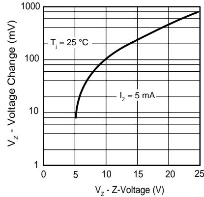
Figure 2. Typical Change of Working Voltage under Operating Conditions at T<sub>amb</sub>=25°C
