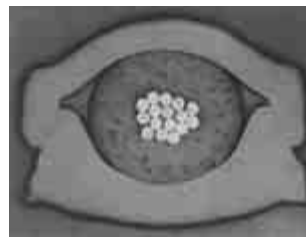
Insulation Crimp Cross Section
