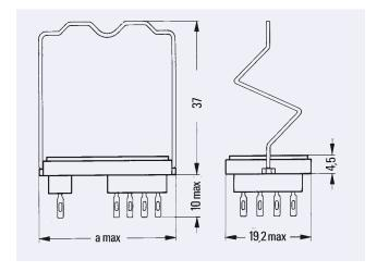
with hold-down spring for cradle relay W
