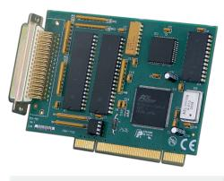
The PCI-PIO is a PCI-compatible half-card which provides digital input/outputs and counter/timers. There are 48 TTLcompatible programmable digital input/outputs available from the board. If the controlling devices are used in handshake mode, the handshake lines are available as interrupt sources.
