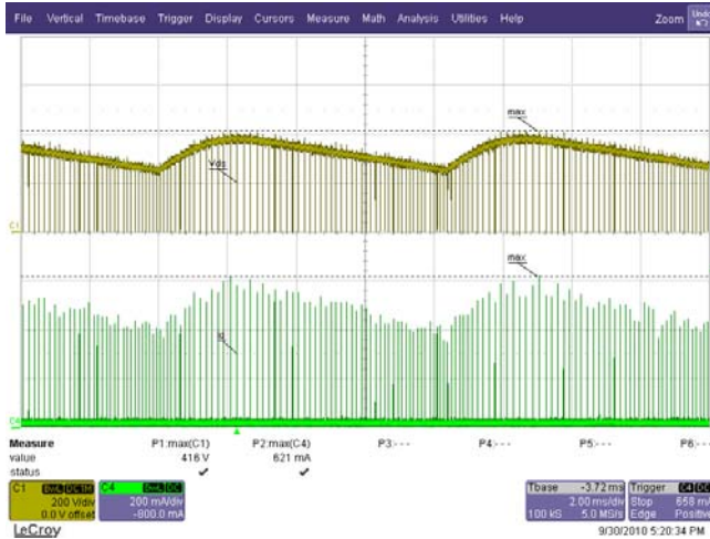
Figure 47 – 265 VAC. Load Shorted. Upper: V_{DRAIN} , 200 V / div. Lower: I_{DRAIN} , 0.2 A / div., 2 ms / div.
