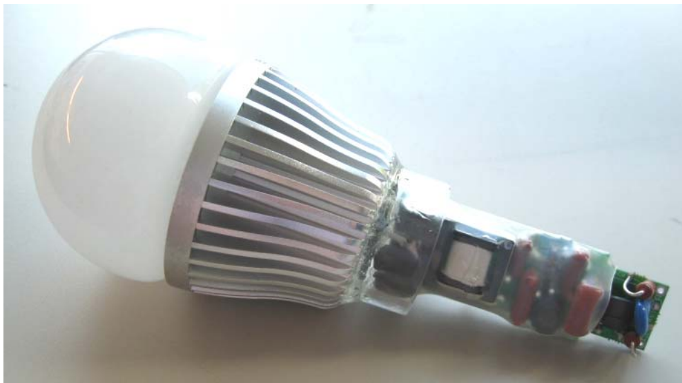
Figure 3 – Example of RD-251 Used in an A19 LED Replacement Lamp (board removed from housing).
