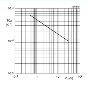
$T_{j}=0~^{\circ}\text{C to }85~^{\circ}\text{C}.$  Fig 3. Temperature coefficient of diode capacitance
