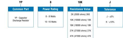
temperatures from -55°C to 350°C. The terminals are designed for quick and easy mounting on capacitors and have a mounting pitch of 22.2 and 31.8 mm. These are wirewound ceramic core resistors designed for voltage balancing of series connected aluminium electrolytic capacitors. These resistors are also suitable for capacitor voltage discharge safety applications in high voltage circuits. Ideally suited for industrial grade capacitors.
