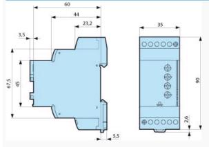
Temperature control relays for lift machine rooms are designed for monitoring the temperature between 5 °C and 40 °C according to standard EN81.
