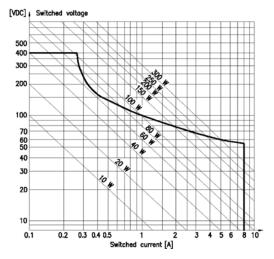
Loads in the range under the curve can be switched safely. The arc will extinguish before the opposite contact makes.
