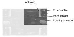
If an inner contact should weld, then the movement of the rotating armature is blocked via the actuator. Open contacts of all four contact pairs remain open.
