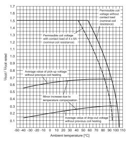
Permissable coil voltages and pick-up and drop-out characteristics at various ambient temperatures.
