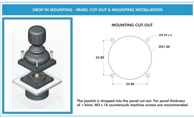
Note: The dimensions shown are for a generic 9000 Series with the third axis R type handle. For specific dimensions of this or any other configuration please refer to Apem.
