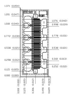
Units: millimeters (inches) Thickness: 0.1016 (0.004)
