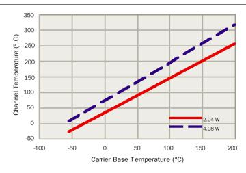
$38\ \mu m$  AuSn solder attach to 0.5 mm CuMo Carrier.
