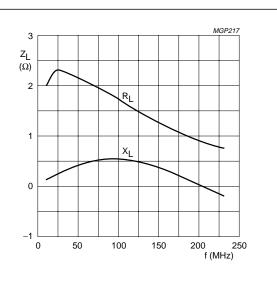
$$\label{eq:GS} \begin{split} & \text{Class-AB operation; } V_{DS} = 28 \text{ V; } I_D = 2 \times 250 \text{ mA;} \\ & \text{R}_{GS} = 536 \ \Omega \text{ (per section);} \\ & \text{P}_L = 300 \text{ W (total device); } T_h = 25 \ ^\circ\text{C}. \end{split}$$
