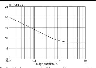
Fig.5. Maximum permissible repetitive rms on-state current  $I_{T(RMS)}$ , versus surge duration, for sinusoidal currents, f = 50 Hz;  $T_{hs} \le 73$  °C.
