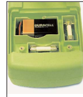
separate battery & fuse compartment
