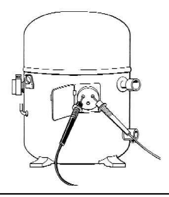
When measuring resistance of a motor, make sure the power is disconnected prior to testing. Set up meter following steps under "Measurement Procedure" on page 16, and proceed with the following:
