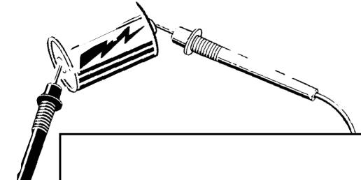
When measuring DC Voltage of a battery, the most accurate reading can be attained by testing the battery under load. To accomplish this, follow steps 1 through 4 shown on page 14 and the following (with the battery in holder and device turned on):
