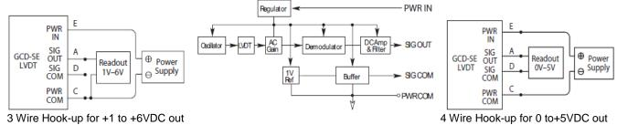
(A through E: Connector pin assignments)
